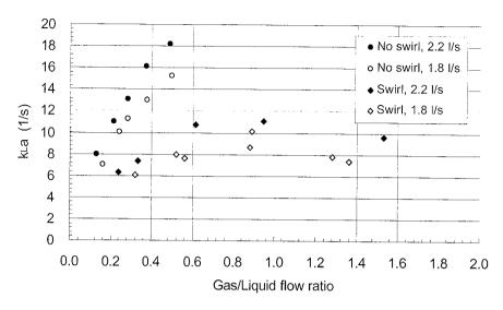
Fig. 6.7 Effect of a swirl device on the local k<sub>1</sub> a-value in the mixing zone
