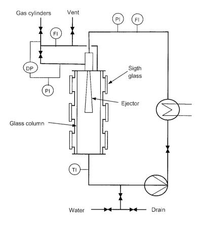
Fig. 3.2 Scheme of the experimental facility.
