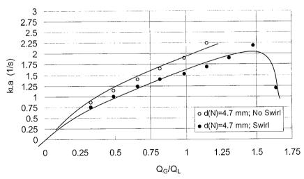
Fig. 5.4 Influence of a swirl device on the volumetric mass transfer coefficient ( $Q_1 = 0.5 \text{ l/s}$ ,  $d_N = 4.7 \text{ mm}$ ,  $L_M/d_M = 2$ , System: water/nitrogen).
