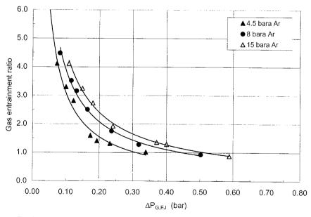
Fig. 3.4 (c) Effect of the reactor pressure on the gas suction rates of ejectors. System: Water-argon ( $Q_L = 5 \text{ m}^3/\text{h}$ )
