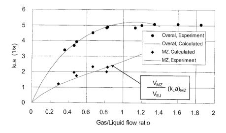
Fig. 6.10 Effective contribution of the mixing zone section to the overall k<sub>L</sub>a value of the straight tube ejector
