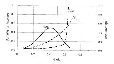
6.8(a) Influence of the d<sub>J</sub>/d<sub>M</sub> ratio on the calculated values of the mixing zone volume, the specific energy dissipation and the energy dissipation rate
