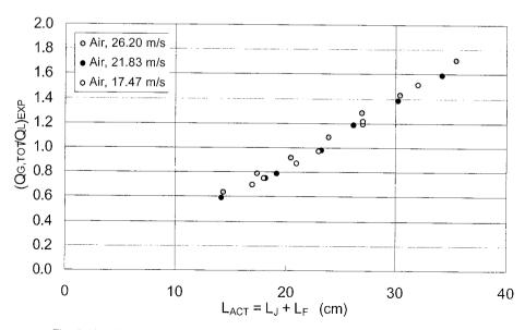
Fig. 2.13 Influence of the actual free jet length (L<sub>ACT</sub>) and jet velocity on the actual entrainment ratio (system: water/air).
