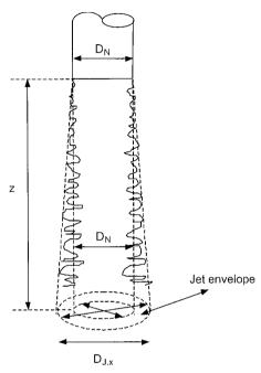
Fig. 2.1 Scheme of the jet envelope mechanism (McCarthy, 1972)
