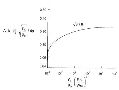
Fig. 2.4 Theoretical dependence of the jet divergence angle on the operating conditions (Ranz, 1958)
