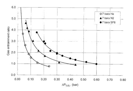
Fig. 3.5 Effect of the gas molecular weight on the gas suction rate of the ejector  $(P_R=0.5 \text{ MPa} \text{ and } Q_1=5 \text{ m}^3/\text{h}).$
