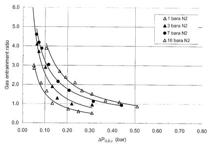
Fig. 3.4 (b) Effect of the reactor pressure on the gas suction rates of ejectors. System: Water-nitrogen ( $Q_L = 5 \text{ m}^3/\text{h}$ )
