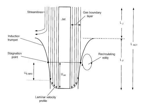
Fig. 2.2 Entrainment of gas film adjacent to the liquid jet (Evans, 1990).
