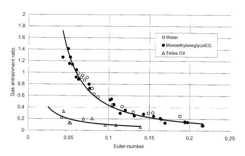
Fig. 3.8 Effect of the liquid physical properties on the gas suction rate of ejectors (Brahim et al, 1984)
