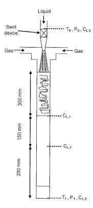
Fig. 6.4 Scheme of the straight tube ejector
