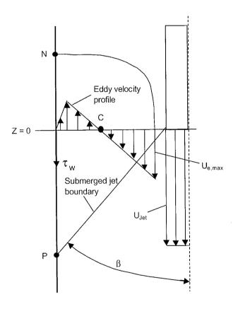
Fig. 6.3 Velocity profile of re-circulating eddy at z = 0 (Evans, 1990).
