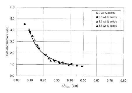
Fig. 3.7 Effect of the solids concentration on the gas suction rates of ejectors. System: water-air and activated carbon particles
