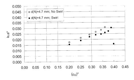
Fig. 5.6  $(k_La)^*_{Ej}$  versus  $(\epsilon_G)^*$ ;  $Q_L = 0.5$  l/s;  $d_N = 4.7$  mm,  $L_M/d_M = 2$  (System: water/nitrogen).
