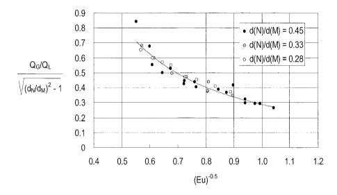
Fig. 3.10 Effect of the mixing tube to nozzle diameter ratio on the entrainment ratio of ejectors (Biswas et al., 1982).
