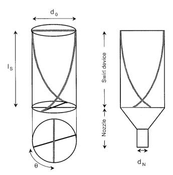
Fig. A 3.1 Geometrical parameters of Swirl device and connection to ejector nozzle.
