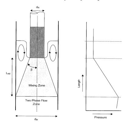
Fig. 6.2 Schematic representation of the mixing zone: Expansion of the two-phase submerged jet.
