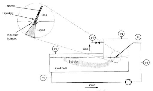
Fig. A2.1 Scheme of experimental facility.
