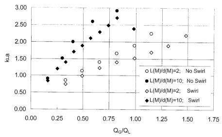
Fig. 5.9 Influence of the mixing tube length on  $k_L a)_{Ej}$  (Q<sub>L</sub>=0.5 l/s, d<sub>N</sub>=4.7 mm, System: water/nitrogen).
