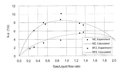
Fig. 6.6(a) Influence  $Q_G/Q_L$  on  $k_La$  in the mixing zone and in the two phase flow zone  $Q_L = 1.8$  l/s (swirl device present in the upstream section of the nozzle)
