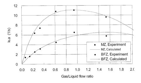
Fig. 6.6(b) Influence  $Q_G/Q_L$  on  $k_La$  in the mixing zone and in the two phase flow zone  $Q_L = 2.2$  l/s (swirl device present in the upstream section of the nozzle)
