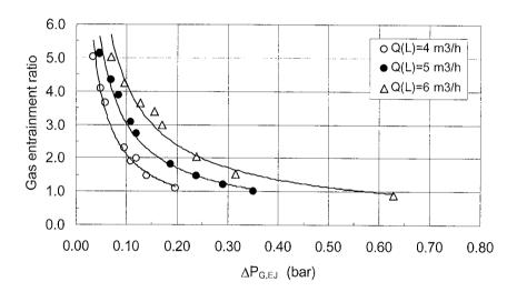
Fig. 3.3 Effect of the jet velocity and the gas phase pressure differential on the actual volumetric gasliquid flow ratio (reactor pressure is 0.5 MPa and the system used was water-nitrogen).
