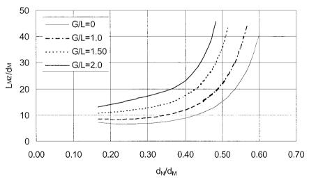
Fig. 6.9 Influence of  $d_N/d_M$  and  $Q_G/Q_L$  on the calculated  $L_M/d_M$ -ratio.
