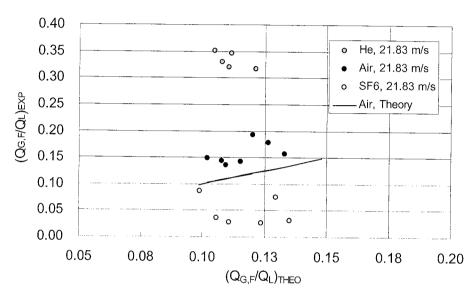
Fig. 2.15 Parity plot of the calculated and the experimental (extrapolated) gas entrainment ratios of the gas film (water/helium and water/SF<sub>6</sub>).
