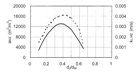
Fig. 6.8(b) Influence of the  $d_J/d_M$  ratio on the calculated values the local mass transfer characteristics ( $k_I$  and a) in the mixing zone.
