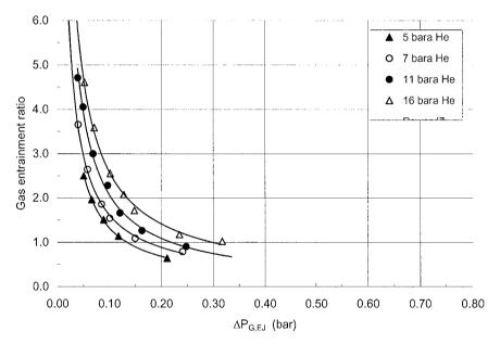
Fig. 3.4 (a) Effect of the reactor pressure on the gas suction rates of ejectors. System: Water-helium ( $Q_L = 5 \text{ m}^3/\text{h}$ )
