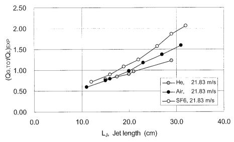
Fig. 2.8 Influence of the gas density on the gas entrainment  $(Q_{G,TOT})$  ratio of plunging jets as function of the jet length  $(L_J)$ .
