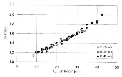
Fig. 2.10 Influence of the jet velocity on the jet stability.
