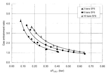
Fig. 3.4 (d) Effect of the reactor pressure on the gas suction rates of ejectors. System: Water-SF<sub>6</sub> ( $Q_L = 5 \text{ m}^3/\text{h}$ )
