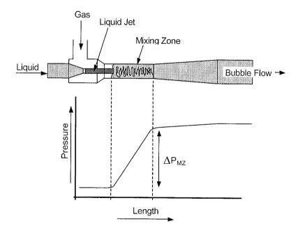
Fig. 6.1 Hydrodynamic conditions inside the ejector and the qualitative change of the pressure along the mixing tube and the diffuser of the ejector.
