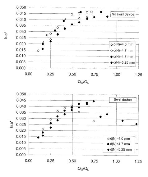
Fig. 5.7 Influence of the nozzle to mixing tube diameter ratio on  $(k_L a)^*_{Ej}$ ; (a) Ejector without swirl device and (b) ejector with swirl device.  $(L_M/d_M = 10 \text{ and } d_M = 12 \text{ mm, System: water/nitrogen})$
