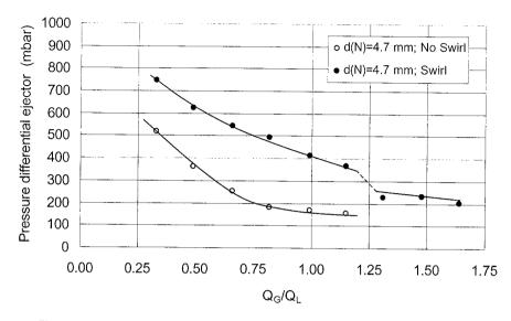
Fig. 5.5 Influence of a swirl device on the gas phase pressure differential (Q<sub>L</sub> = 0.5 l/s, d<sub>N</sub> =4.7 mm, L<sub>M</sub>/d<sub>M</sub> =2, System: water/nitrogen).
