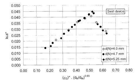
Fig. 5.8 (a)  ${(k_La)}^*_{Ej} \approx versus \ (\epsilon_G)^* \ (d_N/d_M)^{0.65}$  (With swirl, L<sub>M</sub>/d<sub>M</sub> =10 and d<sub>M</sub> = 12 mm, System: water/nitrogen)
