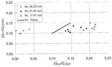
Fig. 2.14 Parity plot of the calculated and the experimental (extrapolated) gas entrainment ratios of the gas film (system: water/air).
