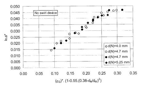
Fig. 5.8 (b)  $(k_L a)^*_{Ej} \approx versus \ (\epsilon_G)^* \ (1-0.55(0.38 - d_N/d_M)^2)$  (No swirl,  $L_M/d_M = 10$  and  $d_M = 12$  mm, System: water/nitrogen)
