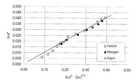
Fig. 5.14  $(k_La)^*E_j$ , versus  $(\epsilon_G)^*(\rho_G)^{0.2}$ ;  $Q_L = 0.5$  l/s,  $d_N = 4.7$  mm,  $L_M/d_M = 2$  (Swirl device present).
