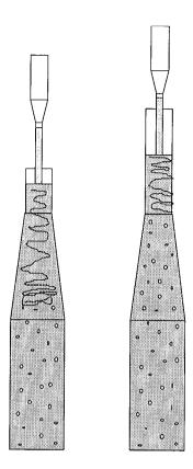
Fig. 5.11 Influence of the mixing tube length on the ejector hydrodynamics (jet velocity and gas-liquid flow ratio are identical).
