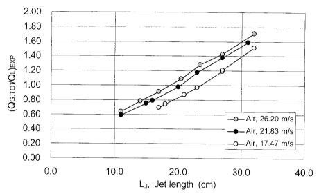
Fig. 2.7 Influence of the jet length (L<sub>J</sub>) and jet velocity on the entrainment rate (Q<sub>G,TOT</sub>). (System: water/air)
