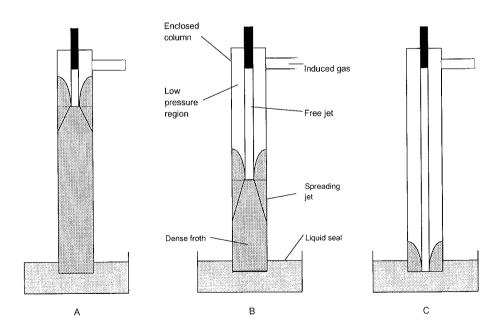
Fig. 2.6 Influence of gas entrainment rate of tube hydrodynamics
