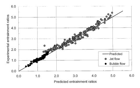
Fig. 3.13 Parity plot of the experimental and predicted (Eqs. (3.17) and (3.18)) gas entrainment ratios.
