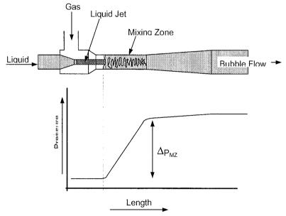
Fig. 1.1 Schematic representation of a gas-liquid ejector.
