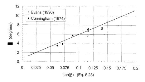
Fig. 6.5 Comparison between measured and predicted jet angle values
