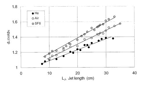
Fig. 2.9 Influence of the gas density on the jet stability.
