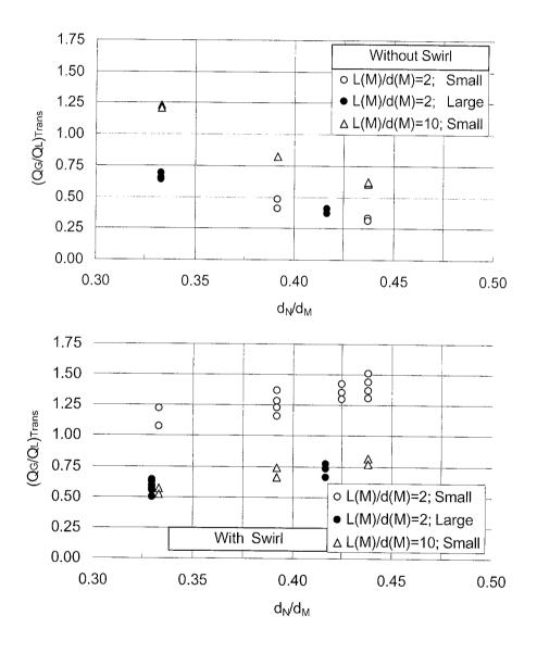
Fig. 5.3 Influence of the geometrical parameters on flow regimes in the ejector: (a) without swirl device and (b) ejector with swirl device
