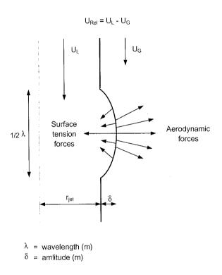
Fig. 2.3 System of forces acting on a slightly disturbed gas-liquid interface.
