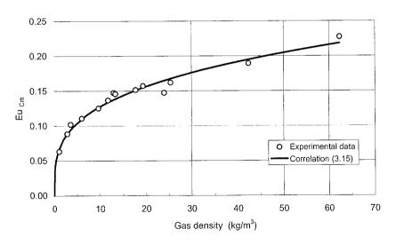
Fig. 3.12 Effect of the gas density on the critical Euler-number
