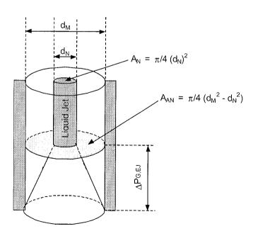
Fig. 3.9 Schematic representation of the mixing zone and of the forces which determine its location in the ejector.
