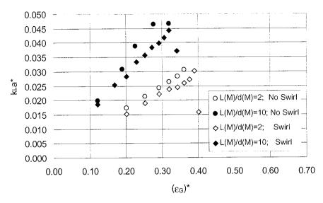
Fig. 5.10 Influence of the mixing tube length on (k<sub>L</sub>a)\*Ej. (d<sub>N</sub>=4.7 mm, System: Water/Nitrogen).
