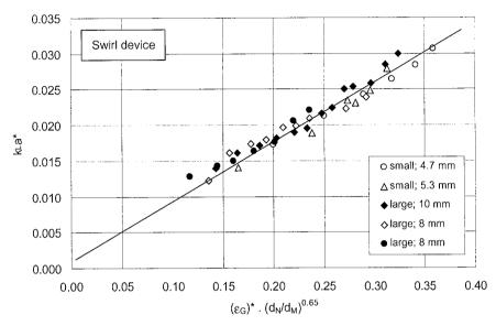
Fig. 5.12 Overview of experiments performed with the standard ejector and with an ejector geometrically scaled up by a factor of 2, both with swirl device in the nozzle (LM/dM = 2),
