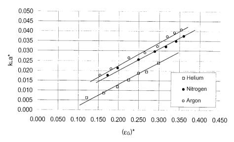
Fig. 5.13 Influence of the gas density on the volumetric mass transfer coefficient of a standard ejector.
