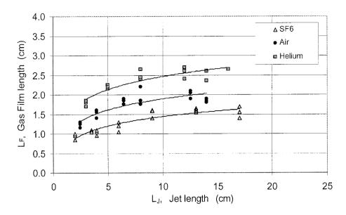
Fig. 2.16 Effect of the physical gas properties on the gas film length
