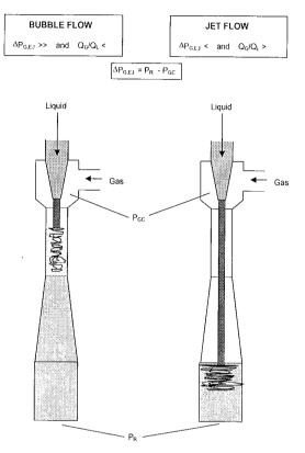
Fig. 3.1 Effect of the gas phase pressure differential on the gas suction rates and the hydrodynamics of the ejector.
