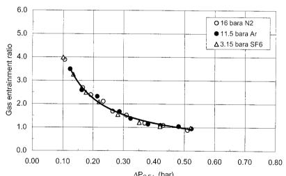
$\Delta P_{G,EJ}$  (bar) Fig. 3.6 Effect of the gas density on the gas suction rates of the ejector (Q<sub>L</sub>=5 m<sup>3</sup>/h)
