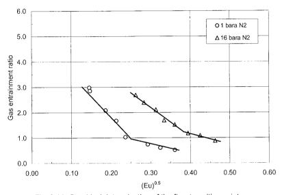
Fig. 3.11 Graphical determination of the flow transition point
