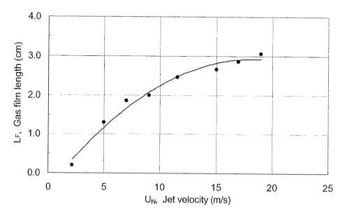
Fig. 2.12 Influence of the jet velocity  $(U_N)$  on the gas film length  $(L_F)$  (Kusabiraki (1990)). (System: Water/air)
